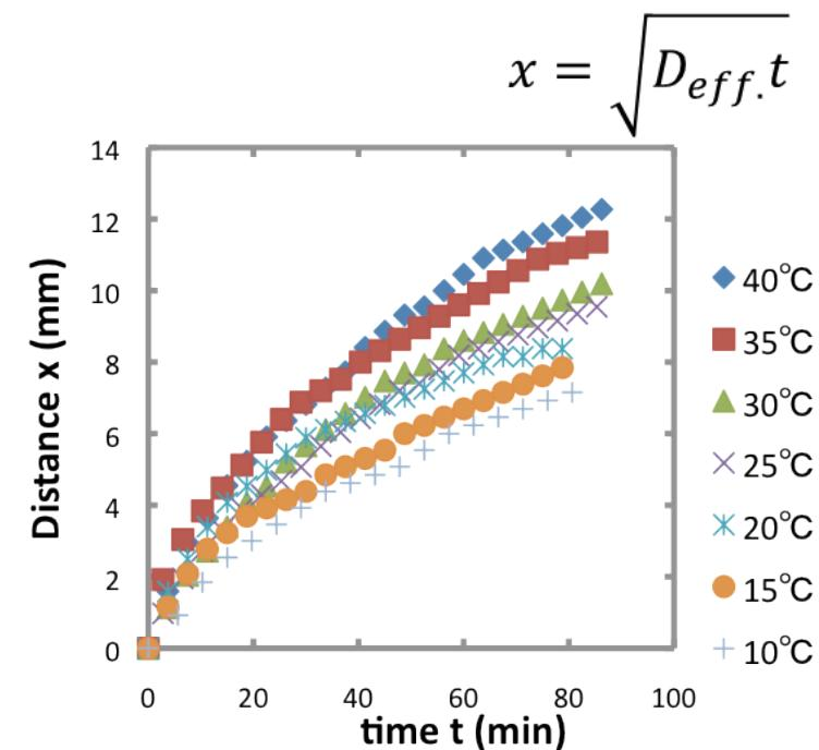
As quenched temperature is increased, the effective diffusion coefficient of precipitation band is larger in a ring pattern
